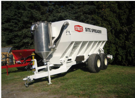
Spreader with high capacity filter can
