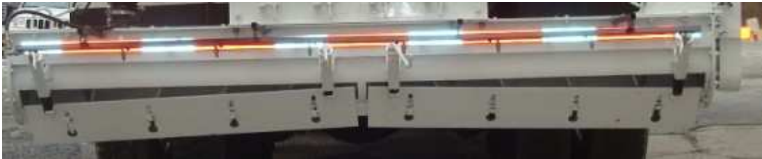
Openings should be wider at the outside of the auger
