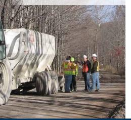
rilling for natural gas in the Marcellus shale region of northern Pennsylvania has increased traffic of heavy loads on small rural roads. Because of the depth and nature of the gasrich shale formation, hydraulic fracturing is being used to release the gas. Each 5-acre drill pad requires about 1,500 trips of 80,000-pound water trucks to open the first well, and 1,000 trips for each additional well. A pad can support up to eight wells.
