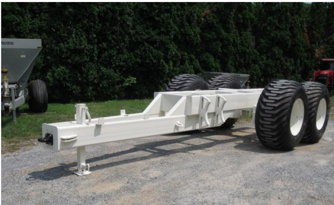
The redesigned floater trailer for the Stoltz SS-2518 cement spreader is pictured here without the spreader body. Already known for its ruggedness and durability, the latest version is 40 percent stronger with its fully welded structural tube steel framework.
