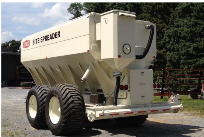
The 27-ton Stoltz SS-2518 spreader is designed for pneumatic filling. Its 300-element low dust filter offers excellent dust control. Operators do not have to climb onto the roof to maintain the filter, an added safety feature.
