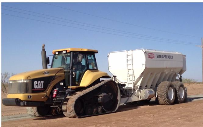
The versatile Stoltz SS-2518 spreader has an optional engine that allows it to be used with vehicles that do not have a power take off (PTO). It can easily handle and distribute a full tanker load of Portland cement under the most severe operating conditions.
