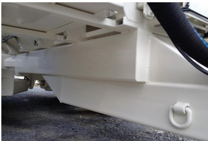
Evident in this close-up view of the redesigned floater trailer, the Stoltz SS-2518 site spreader features a fully welded unibody construction that contributes to the outstanding use record for Stoltz spreaders. Every inch of hopper, frame and attachment points are welded.
